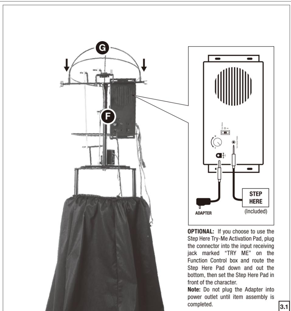
**OPTIONAL:** If you choose to use the Step Here Try-Me Activation Pad, plug the connector into the input receiving jack marked "TRY ME" on the Function Control box and route the Step Here Pad down and out the bottom, then set the Step Here Pad in front of the character.
