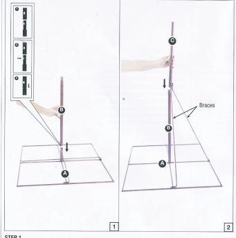
Attach the (B) Support Pole to the (A) Base by aligning the quick-connect push buttons into the pre-drilled holes as shown in Figure 1.
