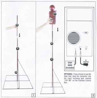
Attach the other (B) Support Pole to the (C) Support Pole with slots by aligning the quick-connect push buttons into the pre-drilled holes as shown in Figure 1.
