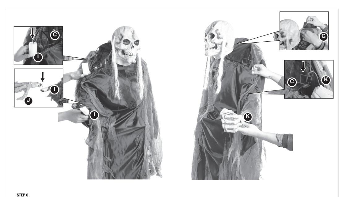
Slide the (I) Right Arm up through the right sleeve and slide the forked-hook into the right "shoulder" slot housing on the (C) Torso Frame. Set the (J) Right Hand into place by sliding the forked-hook into the "wrist" slot housing on the end of the arm. Now, slide the (K) Left Arm up through the left sleeve and slide the forked-hook into the left "shoulder" slot housing on the (C) Torso Frame as shown.
