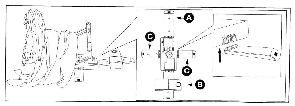
STEP 3 Attached legs (A) (B) (C) by sliding into the groove from the bottom of the base up until snapped into place.
