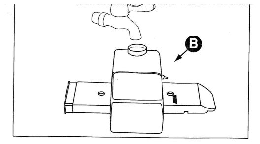
**STEP 2** Fill water bottle and secure cap (B). Make sure the cap is tight to prevent leakage. Note: do not over tighten cap.
