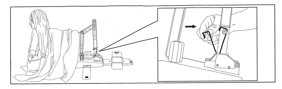
**STEP 4** Lift Character until poles are vertical and attach 2 springs as shown.
