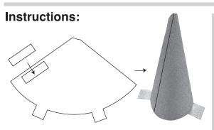
1. Stick one of the double-sided adhesive foam rectangles to the edge of the paper horn piece. Curve the paper to form a cone shape, overlap the edge over the adhesive foam, and press to adhere together.
