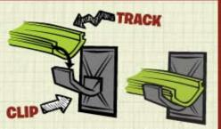
The Velcro®-like material on the clips and board grip together for a tight hold.
