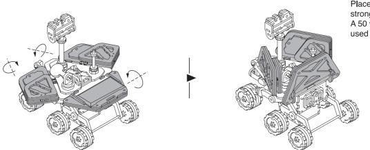
Place your rover in direct and strong sunlight to watch it move. A 50 watt halogen light may be used for indoor use.
